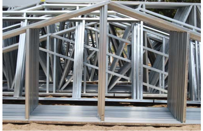
CFS weighs one-third less than wood studs and has the dimensional stability to maintain its structural integrity over the long term.
