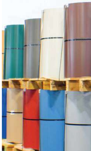
Coatings are for more than just aesthetics. They provide a protective barrier between the elements in the environment that cause corrosion and the readily degradable steel. PHOTO COURTESY OF MILL STEEL.
