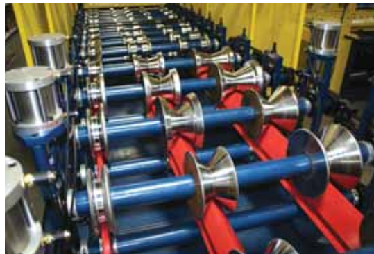
Trim roll former dies. PHOTO COURTESY OF METAL ROLLFORMING SYSTEMS
