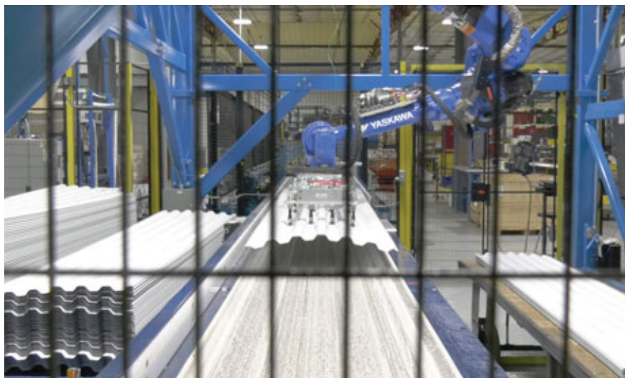
Automated stacker preparing cut and formed metal. Material will be sent to final assembly afterward. PHOTOS AND ADDITIONAL INFORMATION FROM KELLEN ANDERSON OF TRAC-RITE.
