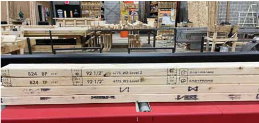
EstiFrame's automated marking system prints blueprints directly onto the framing members.
