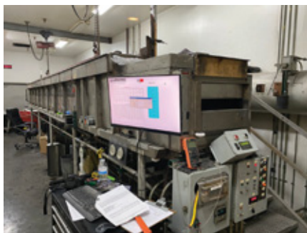
The Dolly Varden T&G rating allows for installation where a Class A is required. At left is the machine used for the “Steiner Tunnel” test method.
