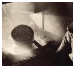
Maze begins making hand-dipped Zinclid™ hot-dip galvanized steel nails
