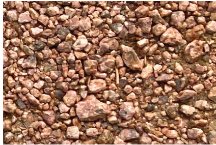
Crushed red granite.
