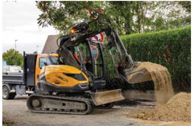
From a single position, a crawler skid excavator can dig then swing up and dump into a truck — all within an incredibly compact 9-foot (2.7-meter) radius.
