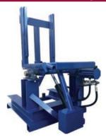
The Four Star Coil Upender is an economical solution to safely tip coils. Functioning only with a hydraulic cylinder and needle valve, it requires no electric or hydraulic hookup, making it very portable with a forklift or pallet jack. It has undergone extensive testing to ensure its safety and efficiency.
