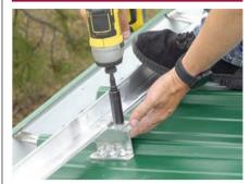
VersaBracket is a bottom-fixed, metal roof bracket designed for mounting ColorGard, solar PV, and other utility mountings to exposed fastened profiles. VersaBracket features a 1" mounting slot on the top flange for adjustability and fastens through the roof, into the deck or structure. Factory-applied butyl sealant ensures speedy installation and lifetime performance.
