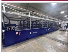
Bradbury Rollforming Line to produce interlocking wall panels features a coil car, 20,000 lb stock reel, roller straightener, and a hydraulic punch/ notch/cutoff system before material enters the 16-pass rollformer. With Bardie Cartridge technology for automatic gauge adjustment, D-2 roll tooling, and a servo-driven Anti Flare Fixture, precision and efficiency are ensured throughout the process.
