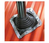
Master Flash Pipe Boots are durable, flexible roof flashings designed to seal around various pipe sizes. Made from high-quality silicone or EPDM, they provide a watertight seal that accommodates roof expansion and contraction. Ideal for HVAC, plumbing, and electrical applications, they resist weather, UV, and extreme temperatures for long-lasting performance.
