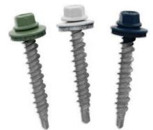
The "PG" woodscrew fastener attaches metal panels to wood-frame applications. It's available in 20 colors and features a #11 Hi-Lo Thread, resulting in better strip to set ratio. The 1/4" hex washer head reduces the screw appearance, and the EPDM bonded 5mm galvanized washer creates a superior seal.
