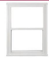
Harmony vinyl windows feature EZv<sup>™</sup> trim and flashing. The exclusive EZ-V<sup>™</sup> system permits installation into a steel-clad building with a fully trimmed panning frame that accommodates the raised ribs of the building skin. Designed for 1" nominal rib height steel, EZ-V<sup>™</sup> reduces labor, is leak-free, paintable, and needs no J-Channel.
