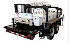
The SSQ II MultiPro features 16 quickchange profiles and can be used inplant or on the road. Change tooling in 45 minutes or less with one person and one wrench. Available with angle cutting and notching functions and with manual control or the option to upgrade to the UNIQ Automatic.
