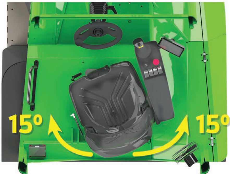
A swiveling forklift seat provides the operator better visibility with reduced fatigue and strain to reduce accidents.
