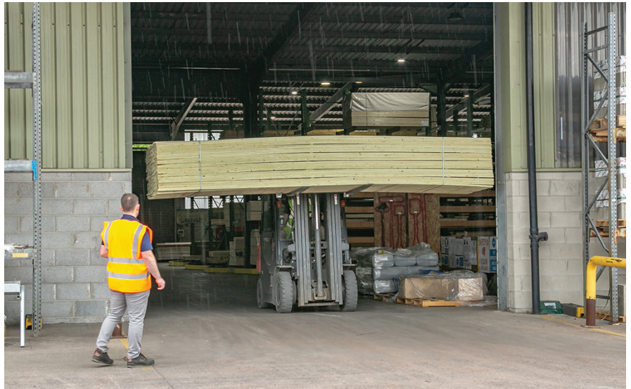
This is an example of a dangerous practice that can cause tipover. OSHA standards mandate keeping the load as close to the ground as possible during travel to prevent an accident.
