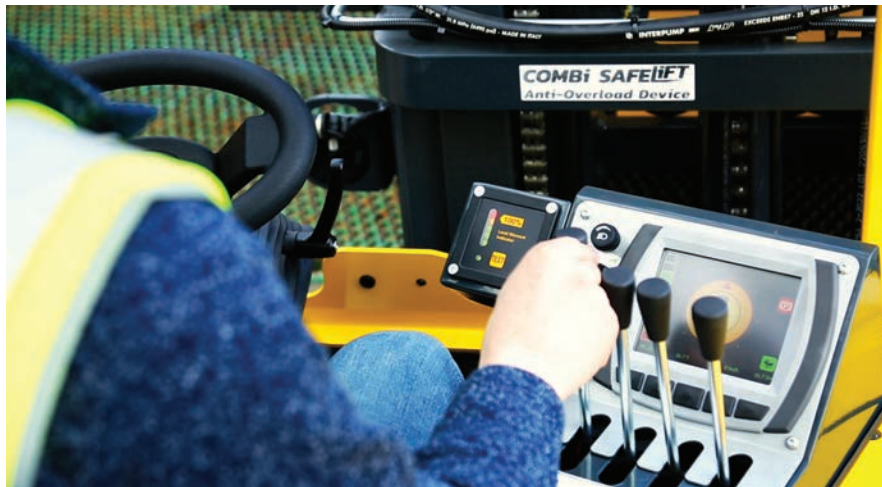
An anti-overload device enables the operator to avoid overloading. If the strain gauge detects an overload situation, it will trigger an audible alarm and will disable lifting.
