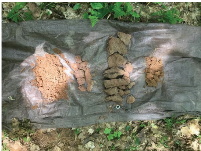
The soil layers from a single soil analysis hole has been separated into four distinct types.
