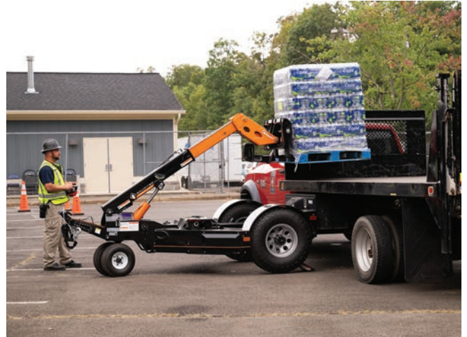
Equipter's Tow-A-Lift Towable Forklift can move materials across landscaping without damaging it.
