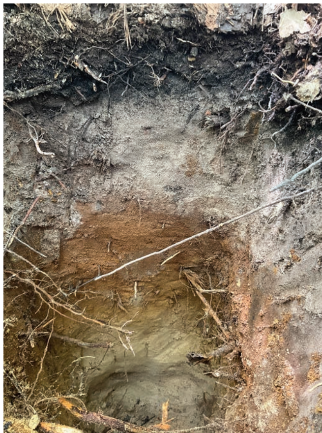
A typical soil analysis hole is about six feet deep. That's the depth that soil maps extend, which is deeper than some foundations. It's not uncommon to encounter several layers of different materials when digging, and these materials will all act differently under load and with the addition or subtraction of moisture.
