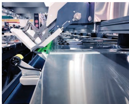
5. Duplex Long Folder bends sheet metal material to part specs.
