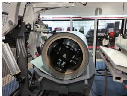
2. Coils are loaded into the Uncoiler and fed into the slitter.
