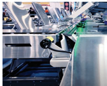
6. Part Handler/Unloader collects finished parts and moves to collection area.
