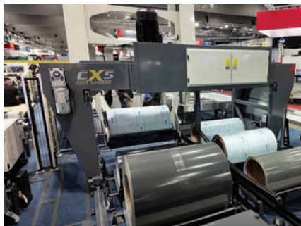
1. CX5 Coil Changer picks coil material according to job specifications.
