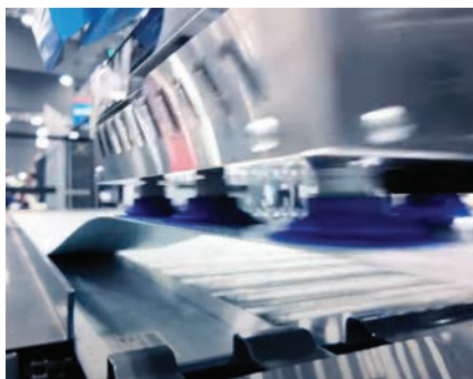
4. Sheet Loader System collects and sorts blanks, then positions into Long Folder.
