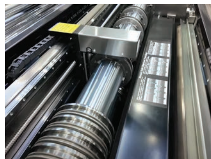
3. Marxman Pro Slitter automatically adjusts blades to the width of the part specification.
