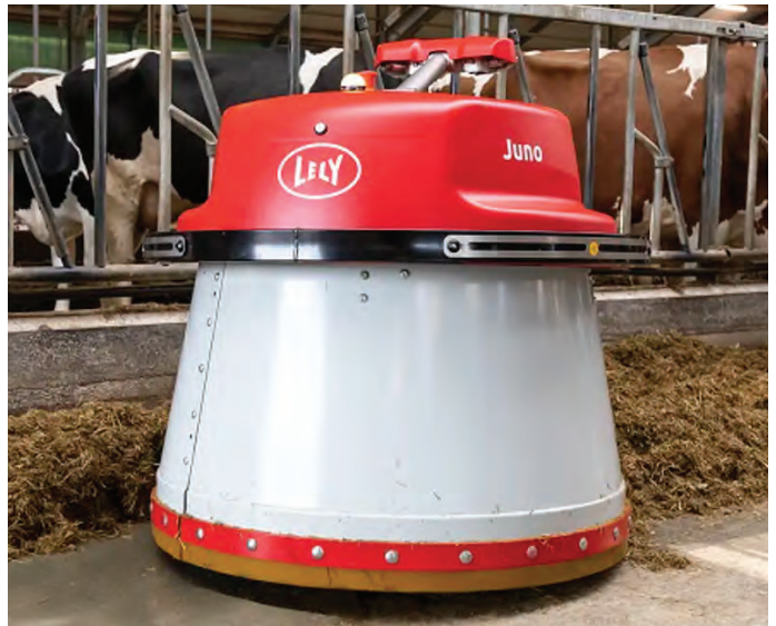
Automatic feed pusher. COURTESY OF LELY JUNO.
