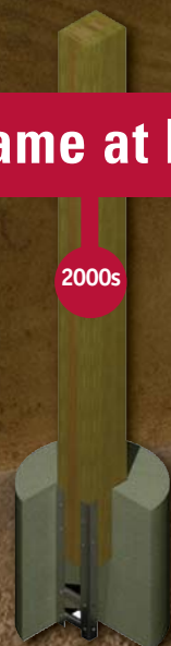
Laminated column with stilts
