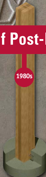
Laminated column in the ground
